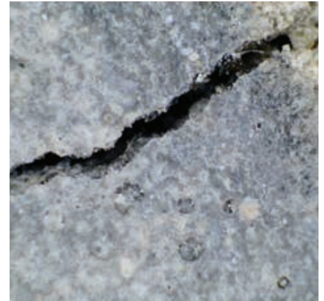
Concrete beam without AQUAFIX (0.5 mm crack)
