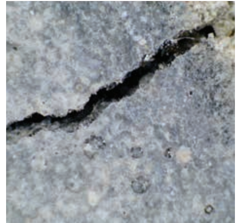
Concrete beam without AQUAFIX (0.5 mm crack)
